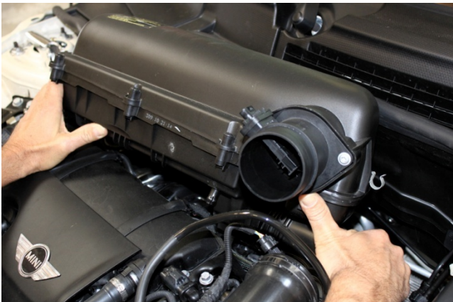
5. Locate fresh air pipe that is attached to air filter box. Disconnect fresh air pipe by rotating the connection counter clockwise and pulling pipe away from air filter box. Remove air filter box from vehicle.
