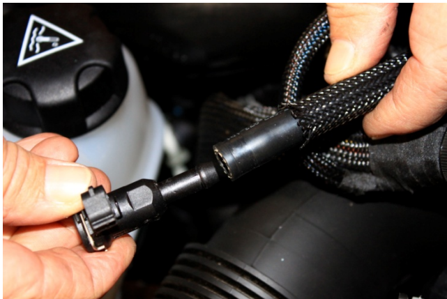
2. Disconnect vent hose on side of turbo inlet pipe, unclip wire connection then cut off hose clamp and remove plastic fitting. NOTE: Some vehicles do not have any hose connected to this fitting. Proceed to disconnecting the sensor connector and cap off the Y adapter's smaller end on step # 17 using the provided vinyl cap.
