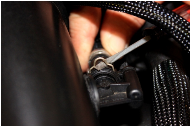
1. Disconnect valve cover breather hose from turbo intake pipe, unclip wire connection then cut off hose clamp and remove plastic fitting.
