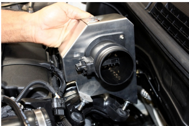
8. Install MAF sensor to NM stainless steel intake pipe bracket using supplied M6 x 16mm button head bolts and M6 nuts. [4mm hex key wrench / 10mm socket or wrench]
