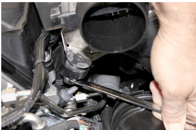
9. Install NM SS bracket onto factory air filter box mounts. NOTE: Make sure rubber grommets are still in place and not attached to bottom of the OE air filter box. From bottom side of mounts, install and tighten using supplied M8 washers and M8 lock nuts. [13mm wrench]
