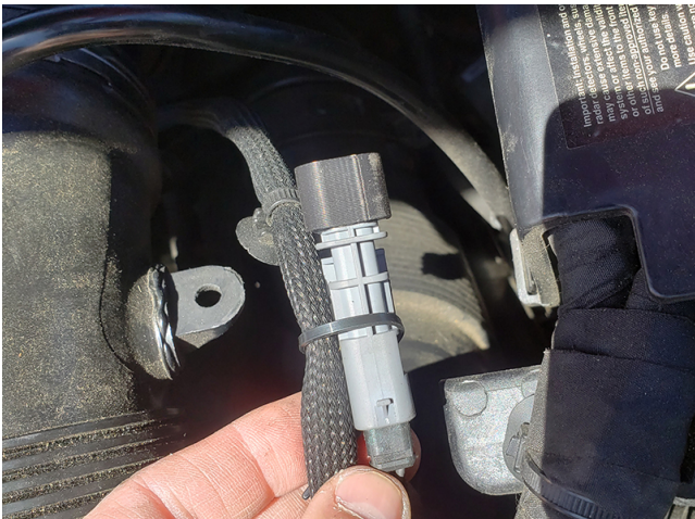
22. Install both heater by-pass connectors and secure them with zip ties to the neighboring wire looms.
