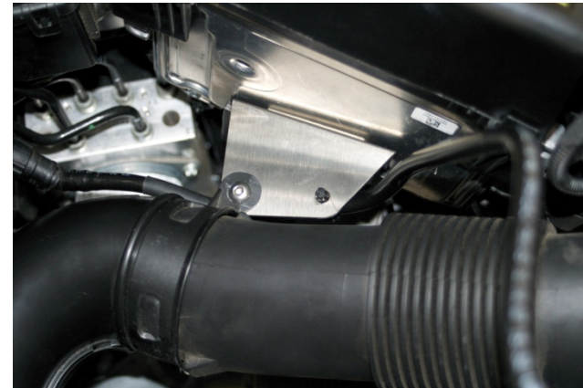
12. 2011-3/2012 Early N18 Attach brake booster line holder to forward mounting hole in bracket. Secure fresh air pipe to rearward mounting hole using supplied M6 x 10mm button head bolt. [4mm hex key wrench]
