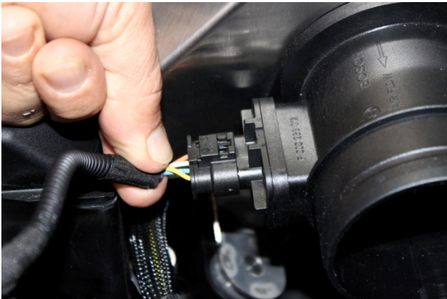
10. Reconnect MAF sensor electrical connector.
