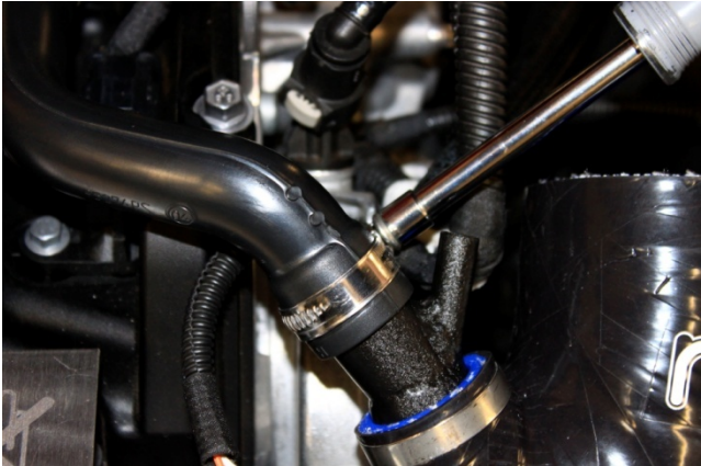
16. Connect breather hose with 25mm clamp supplied.
