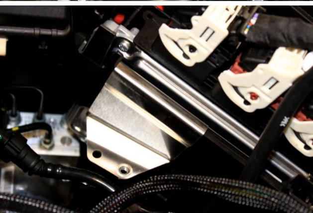
13. 3/2012-UP N18 ECU cover removal: Remove 10mm hex bolt then push inward on tabs to remove cover. Remove protective film from double-sided tape on stainless steel intake duct support bracket. Hook bracket on top edge of black plastic case for ECU, positioning at back corner.
