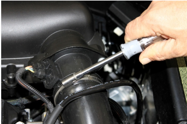
3. Loosen clamp at MAF sensor to turbo intake pipe and disconnect.
