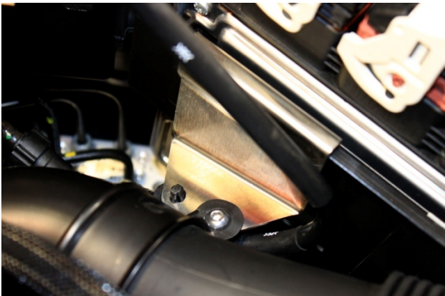
14. 3/2012-UP N18 Attach brake booster line holder to rearward mounting hole in bracket. Secure fresh air pipe to forward mounting hole using supplied M6 x 10mm button head bolt. [4mm hex key wrench]
