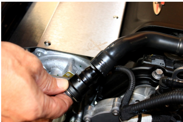
1. Disconnect valve cover breather hose from turbo intake pipe, unclip wire connection then cut off hose clamp and remove plastic fitting.
