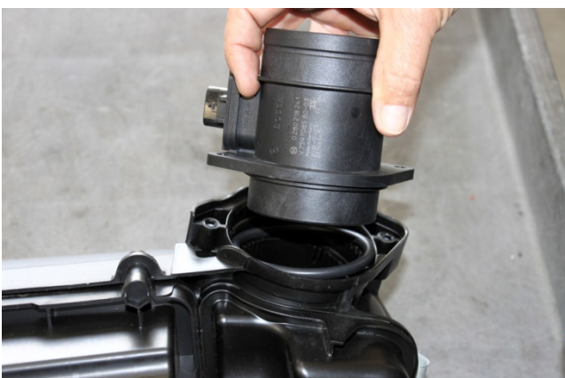
7. Remove MAF sensor from air filter box by removing [2] T30 TORX screws.
