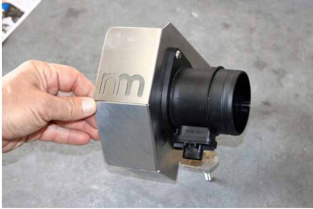
8. Install MAF sensor to NM stainless steel intake pipe bracket using supplied M6 x 16mm button head bolts and M6 nuts. [4mm hex key wrench / 10mm socket or wrench]
