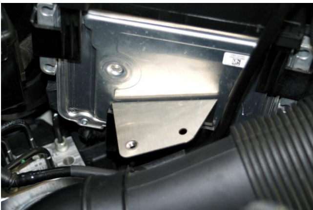
9. 2011-3/2012 EARLY N18 Remove protective film from double-sided tape on stainless steel fresh air hose bracket. Slide bracket down between ECU and black plastic ECU mount, while keeping double stick tape from touching. With bracket pushed all the way down, press against ECU.
