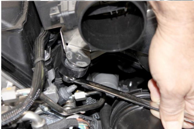
8. Install NM SS bracket onto factory air filter box mounts. NOTE: Make sure rubber grommets are still in place and not attached to bottom of the OE air filter box. From bottom side of mounts, install and tighten using supplied M8 washers and M8 lock nuts. [13mm wrench]
