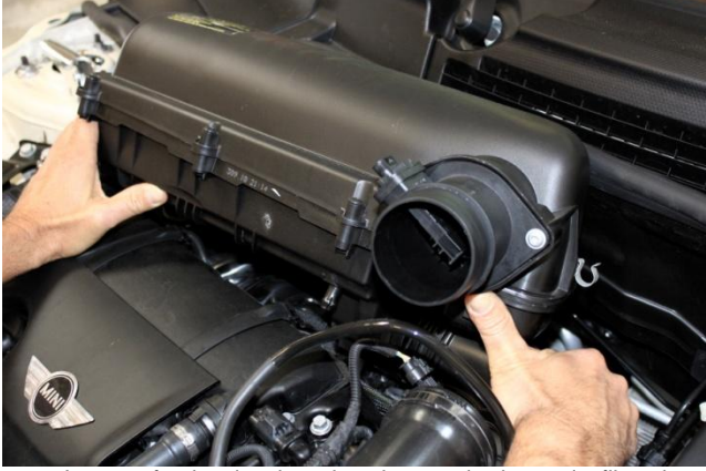
5. Locate fresh air pipe that is attached to air filter box. Disconnect fresh air pipe by rotating the 90° connection counter clockwise and pulling pipe away from air filter box. Remove air filter box from vehicle.
