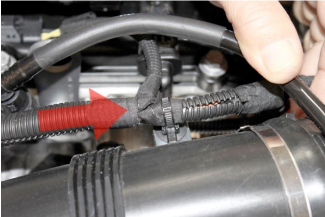
13. Slide MAF wire harness rearward where it attaches with wire tie at turbo intake tube.
