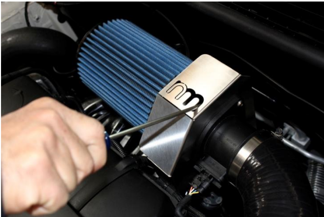
18. Using degreaser or contact cleaner and shop rag, clean inner mounting flange of NM filter. Install NM filter onto MAF sensor and tighten with long skinny screwdriver thru logo cut-out or from back side of bracket.
