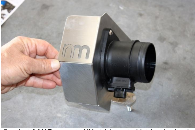
7. Install MAF sensor to NM stainless steel intake pipe bracket using supplied M6 x 16mm button head bolts and M6 nuts. [4mm hex key wrench / 10mm socket or wrench]
