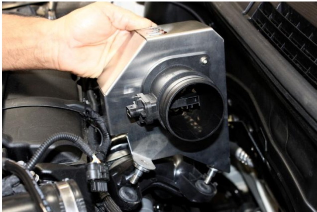
7. Install MAF sensor to NM stainless steel intake pipe bracket using supplied M6 x 16mm button head bolts and M6 nuts. [4mm hex key wrench / 10mm socket or wrench]
