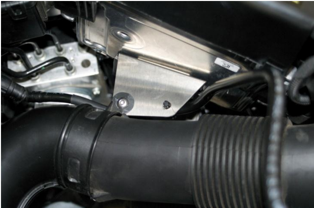
10. 2011-3/2012 EARLY N18 Attach brake booster line holder to forward mounting hole in bracket. Secure fresh air pipe to rearward mounting hole using supplied M6 x 10mm button head bolt. [4mm hex key wrench]
