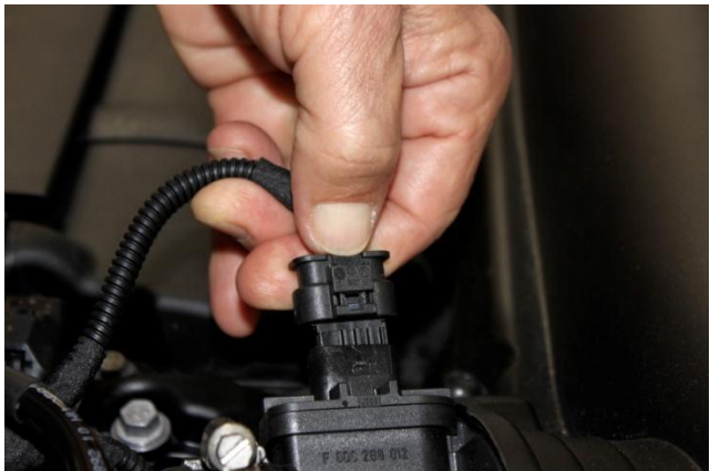
2. Squeeze tab on electrical connector to disconnect from MAF.
