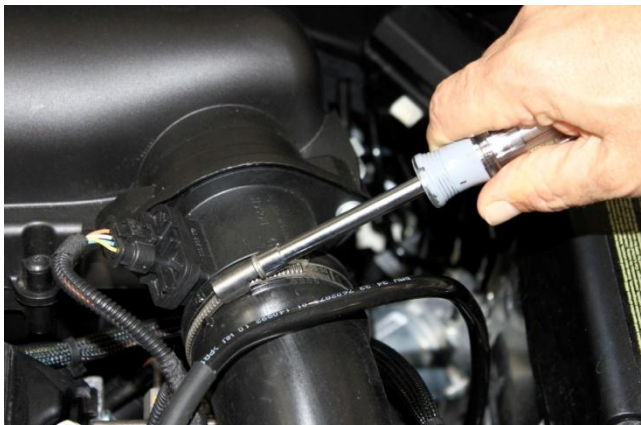
1. Loosen hose clamp at Mass Air Flow sensor (MAF) to turbo intake tube using 7mm nut driver or screwdriver.
