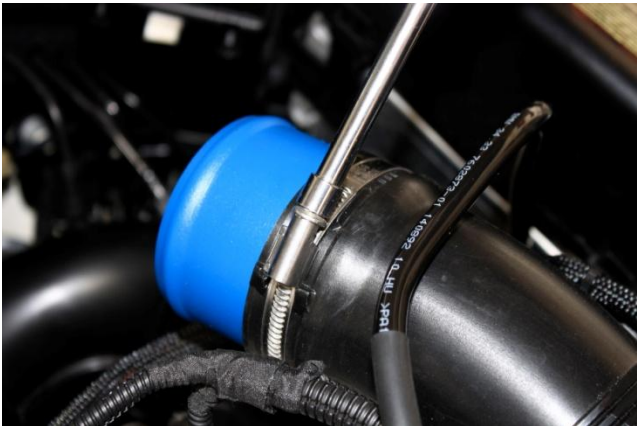
15. Install and fully seat NM connection pipe (non-beaded end) into turbo intake tube then tighten using 7mm nut driver or screwdriver.
