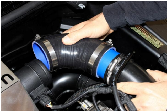
16. Loosely install supplied #44 SS hose clamps onto NM silicone hose. With NM logo on silicone hose facing firewall install onto NM connector first then onto MAF sensor.
