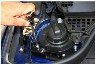
Mount and evenly tighten the left and right NM base plates to strut towers using supplied M8x30mm bolts – torque to 34 Nm (25 ft-lbs).
