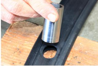
Using hammer, strike a few times to punch through the rubber to the other side.
