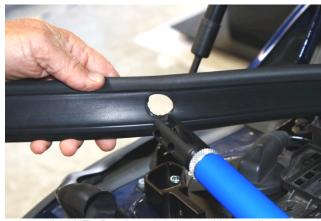
Install NM Tie-Bar through hole in rubber engine bay seal. Repeat for other side.
