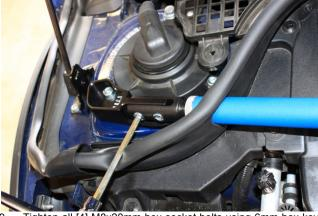
Tighten all [4] M8x20mm hex socket bolts using 6mm hex key wrench.
