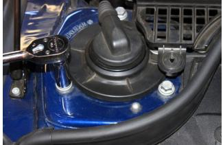
Park MINI on a level surface and remove the [2] forward most 13mm hex bolts on top of each strut tower.
