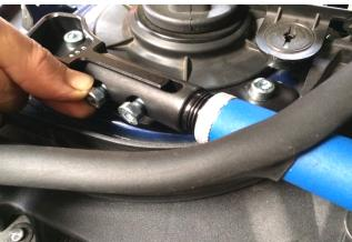
Attach NM Tie-Bar clevis to mounting base plates using [4] M8x20mm hex socket bolts supplied and install rubber engine bay seal at the same time.
