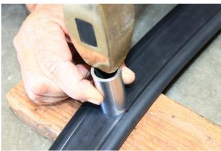
Pull off rubber seal from vehicle and place on a piece of wood. Using punch tool supplied, center over pen mark and center between top and bottom grooves on rubber seal.
