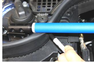
Position NM Tie-Bar on top of rubber engine bay seal and align parallel NM base plate mounting with clevis at both strut towers. NOTE: Center of Tie-Bar will be rotated toward front of vehicle. Then with marking pen draw line directly under centerline of bar onto rubber seal. Repeat at other strut tower.
