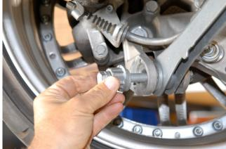
Unbolt and remove outer control arm bolt and adjusting plate using a 16mm socket, then remove control arm.
