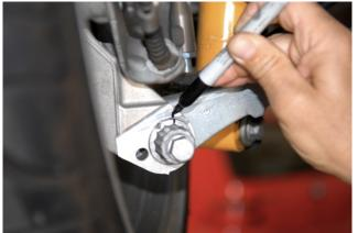
Mark existing location of factory adjusting plate to trailing arm on outer control arm bolt with marking pen.
