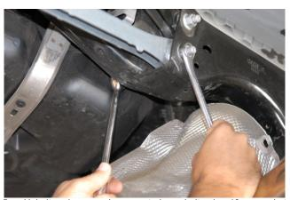
Unbolt and remove inner control arm bolt using 18mm socket and wrench.
