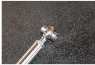
7. Install supplied stainless steel spacers into ball joints.
