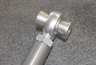
7. **NOTE:** Use wider stainless spacers on inside ball joint that attaches to sub-frame and the narrower stainless steel spacers on ball joint that attaches to outer suspension housing.
