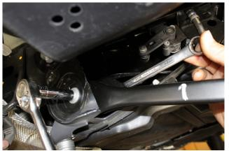
Unbolt and remove inner control arm bolt using E14 Torx or 11mm socket and18mm wrench.  Install and tighten NM Control Arm into inner subframe mount using original bolt and nut. Torque to 100Nm (74ft.lbs). FACTORY ARM LENGTH: 20-3/8" (center to center)
