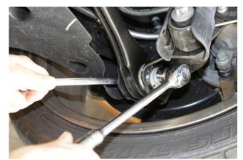
Unbolt and remove outer control are adjusting bolt. Hold bolt head with E14 Torx or 11mm box and wronch and turn put with 18mm acaket
