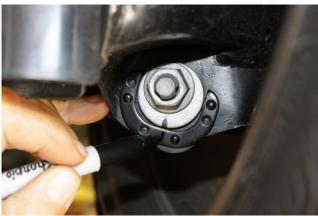
3. Mark existing location of factory adjusting plate to trailing arm on outer control arm bolt with marking pen.
