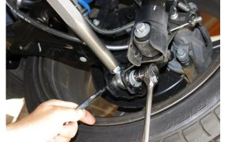
Now install outer NM Control Arm to trailing arm using factory bolt and adjusting plate. Line-up previous made pen mark before tightening. Torque to 100Nm (74ft.lbs).
