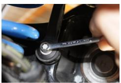
Back out lower end-link mounting bolt about a 1/2" using an E10 Torx or 5/16" wrench or socket. Pull down on anti-roll bar arm due to bushing pre-load and then pull out upper endlink stud from bar. Repeat for other side.
