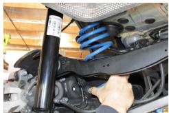
Pull down on trailing arm then pull out suspension spring. Repeat steps #6 and 7 for other side.
