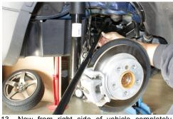
Now from right side of vehicle completely remove original bar.
