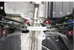
Remove the (4) sub-frame mounting bolts using E14 Torx or 7/16" socket.
