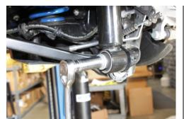
Support with jack under trailing arm and remove lower shock absorber bolt using E20 Torx or 5/8" socket. Lower jack to release spring pre-load.
