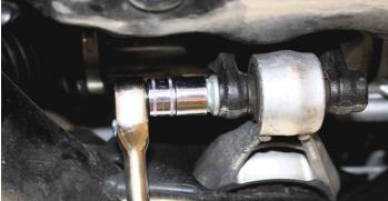
Underneath the vehicle: Remove the 16mm and 18mm hex bolts to remove engine torque arm from sub-frame.
