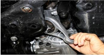
Pull down front of torque arm out of mount, push engine forward then rotate toward transmission and pull out from sub-frame.
