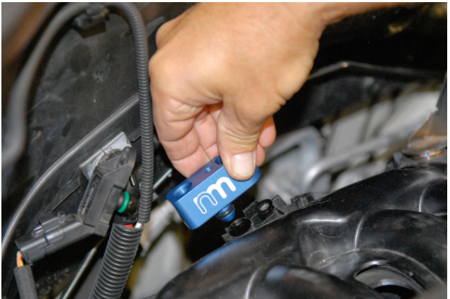
7. Lightly grease “O” ring on NM Boost Sensor Tap and install onto manifold.
