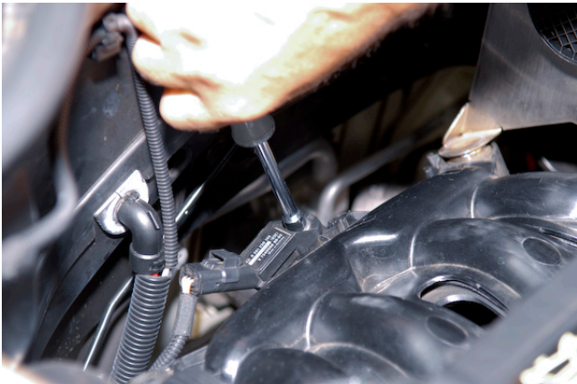
5. Located on back side of intake manifold, remove screw that retains MAP (manifold absolute pressure) sensor using an 8mm Nut Driver or 8mm Socket.
