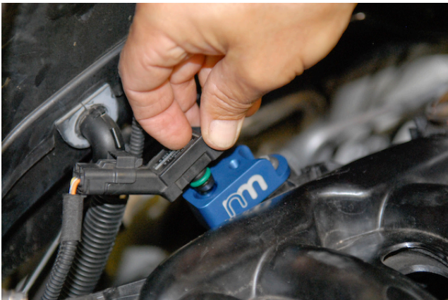
9. Install MAP sensor into NM Adapter, lightly grease “O” ring.
