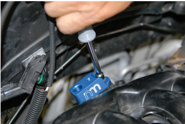
8. Using original screw tighten NM Boost Sensor Tap.
