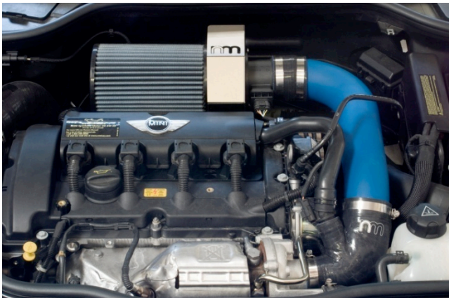
4. If you have NM Hi-Flow Induction Kit just remove filter.
