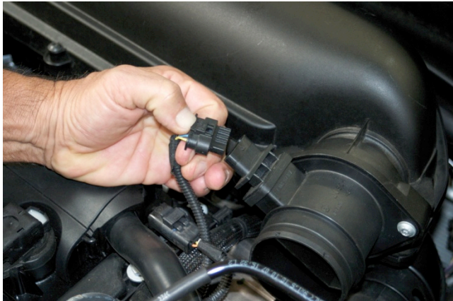
2. Disconnect electrical connector from MAF.
