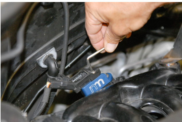
10. Using supplied M6 x 10mm screw, tighten MAP sensor to NM Boost Sensor Tap.
