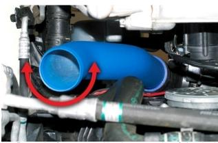
Rotate pipe for correct position, bottom opening of pipe should be parallel to the ground and there should be no interference with any other vehicle components.
