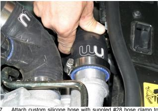
Attach custom silicone hose with suppled #28 hose clamp to turbo; do not tighten at this time. Temporarily remount coolant tank. NOTE: Coolant hose runs above lower pin mount.
