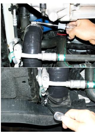
13. Now tighten 90° silicone hose clamps (7mm hex). Double-check pipe for proper clearances from top to bottom.
