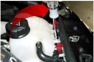
Remove 8mm hex screw that retains coolant reservoir tank. Rotate back side of tank up to release lower pin mount, then lift tank off top retaining tabs. Lay tank to the side.
