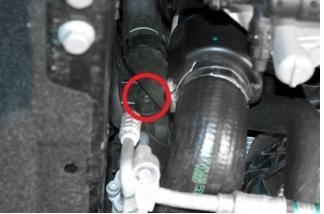
5. From underneath the vehicle, remove the T-25 Torx mounting screw that holds intake muffler to radiator fan shroud.
