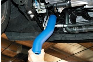
From underneath vehicle install aluminum pipe (longer straight section goes up). Use WD-40 on pipe ends for easier fitment.
