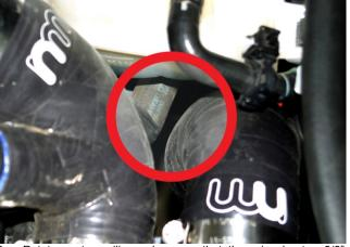
Rotate custom silicone hose so that there is about a 3/8" clearance between it and the coolant hose. Then tighten hose clamp (8mm hex).
