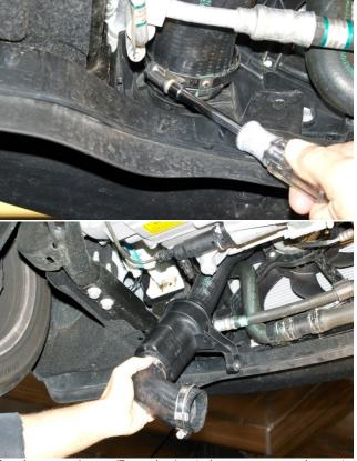
Loosen clamp (7mm hex) at lower pressure hose to intercooler; now remove hose and muffler downward from vehicle
