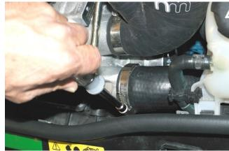
Loosen turbo discharge hose clamp (7mm hex) and disconnect hose from turbocharger.
